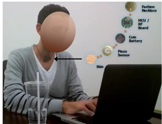
Fig. 1. This figure shows a subject wearing the necklace while working. The necklace comprises a piezoelectric sensor, coin battery, MCU/RF board and a fashionable cover, while maintaining contact between the sensor and skin.
