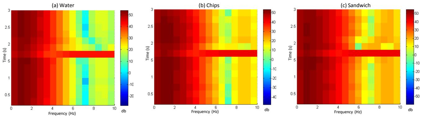
Fig. 3. Figure a shows the spectrogram for a water swallow over a 3 second window. Figure b and Figure c show the spectrogram for chips and sandwich, respectively. The distinction between water and solid is evident in the spectrogram which exhibits lower frequency components, while the sandwich exhibits more higher frequency components. Finer differences are captured when we extract statistical features on each spectrogram.
