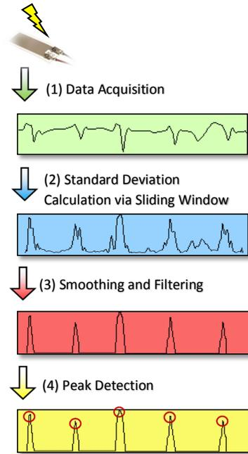
Fig. 2. This figure shows the swallow detection process, whereby a sliding window is applied to the signal to generate a waveform representing the standard deviation of the signal, after smoothing, peaks are detected and identified as potential swallow regions.
