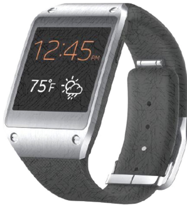
Fig. 2. The Samsung Galaxy Gear is the chosen hardware platform, which runs Android 4.2.1 and features an 800 MHz ARM-based processor.
